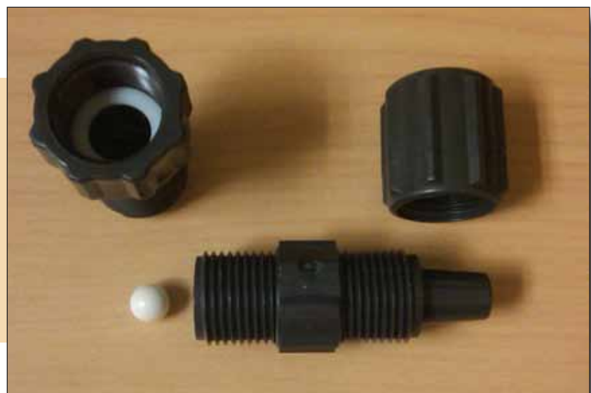
An injector check valve was used on the sodium metabisulfite line as a backflow prevention device.
